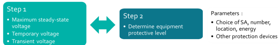
FIGURE 77: Simplified view of procedure for the determination of voltage withstand levels coordination procedure proposed by the IEC 60071-11
